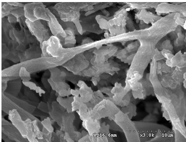
Fig. 9. SEM microphotograph showing the surface of a white alteration (sample 80-CTM:alt) observed on the left of panel 2. Fungal hyphae encrusted with small calcium oxalate crystals are observed (dotted segment 10 \mu m).
